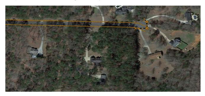
The orange lines in the above picture indicate roadside ditches which are structurally maintained by the MWA. The runoff enters the ditches and flows downstream to the cul-de-sac where there are catch basins and pipes indicated by the orange/black lines and circles owned and maintained by the MWA.
