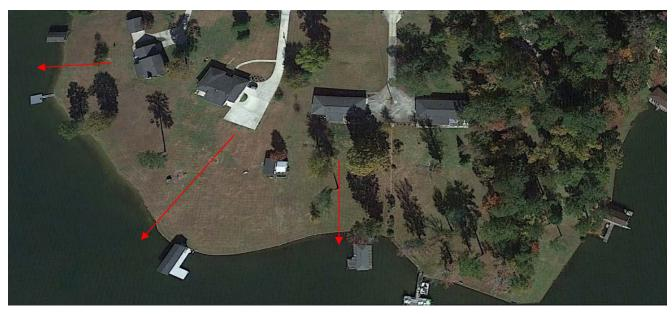
The stormwater runoff from these properties drains directly to the lake thus entering no infrastructure maintained by the MWA.
